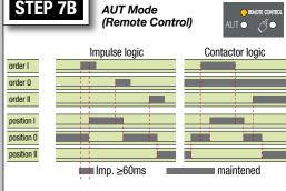
To enable control, close contact 312 with 317. For contactor logic bridge contact 316 with 317. To operate: close the contact corresponding to the desired position. To force the product to 0 position "OFF" bridge
